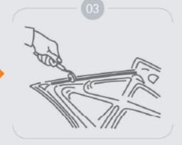
Apply pressure with roller and sliding it
