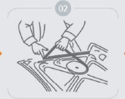
Remove release paper of sealing tape and attach to panel work surface
